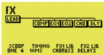
It is simplest for you to sing through the VoicePrism and alter the softknob settings in order to get a feel for how the different parameters affect the sound. There is an abbreviated name above each softknob to let you know which parameter you are adjusting, the current setting is displayed below the parameter name. For a full description of each parameter refer to the VoicePrism User Manual.
