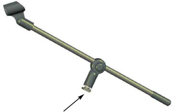
6. Lift the lid on VoiceSolo XT, and while holding it open, slide the Mic Boom Mount attachment, on the boom into slot on top of the monitor and let the lid close.
