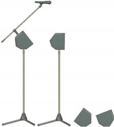
1. Separate the boom from the stand by unscrewing the boom from the vertical shaft of the microphone stand. To do this, tighten the clutch you use to raise and lower the stand first. This makes it easier to unscrew the boom section. Hold the base of the stand with one hand and turn the boom counterclockwise (looking down from the top) with the other hand.
