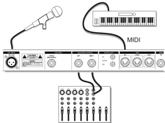
Demo setup #1: Mic input and analog mixer
